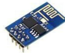
Figure 3. ESP8266 Wi-Fi Module
