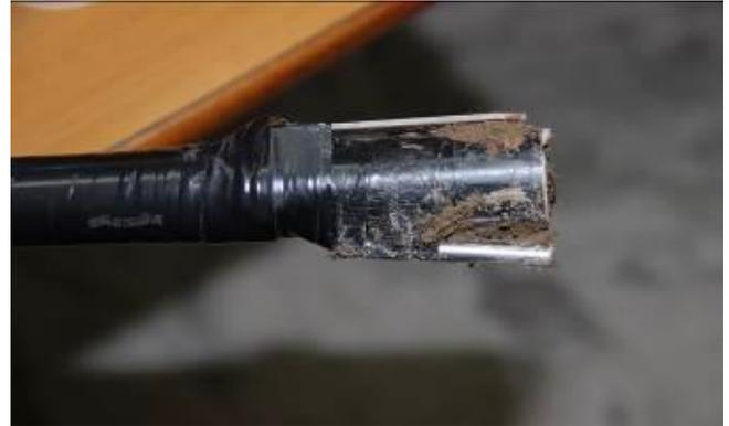
Figure 15. Soil Moisture Sensor and Temperature Sensor Mounted on IoT Agriculture Stick.
