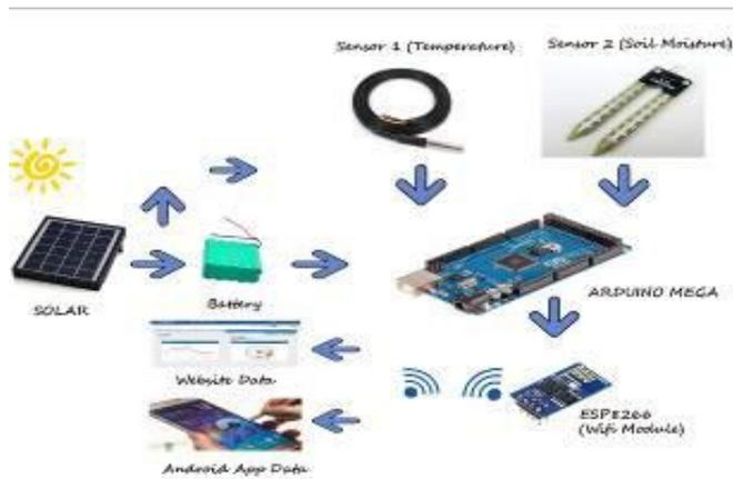
Figure 13. Overall System Working of “Smart IoT Based Agriculture Stick”
