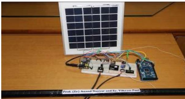
Figure 14. Complete Agriculture IoT Stick Monitoring Temperature and Humidity
