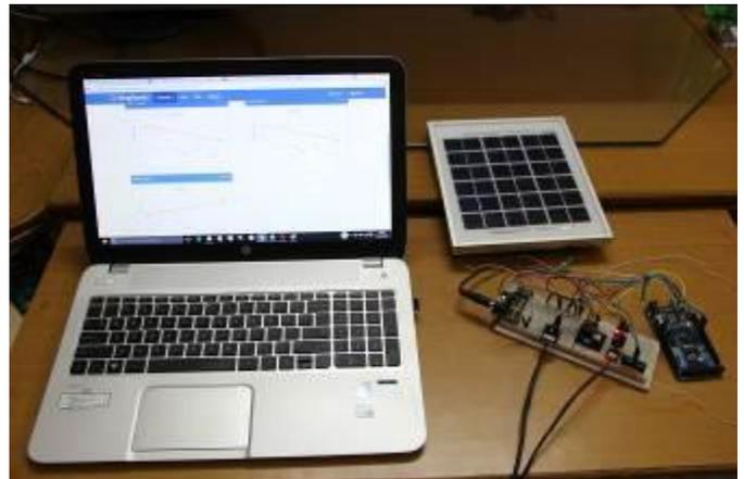
Figure 17. Complete system with Arduino Board, BreadBoard and Laptop giving results using ThingSpeak.com website
