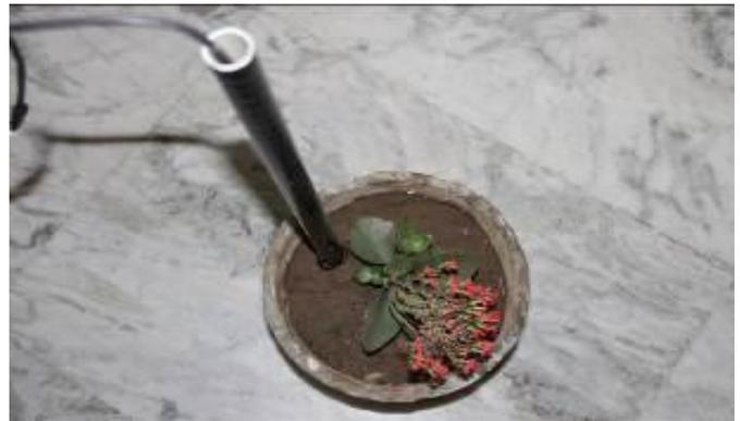
Figure 16. Stick Mounted with Sensors in Flowerpot giving Live Data of Temperature and Moisture.
